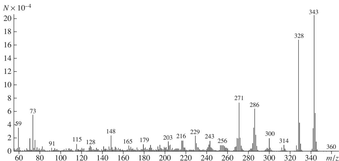
Fig. 4. Mass spectrum of the trimethylsilyl derivative of desomorphine (retention time, 18.897 min).
