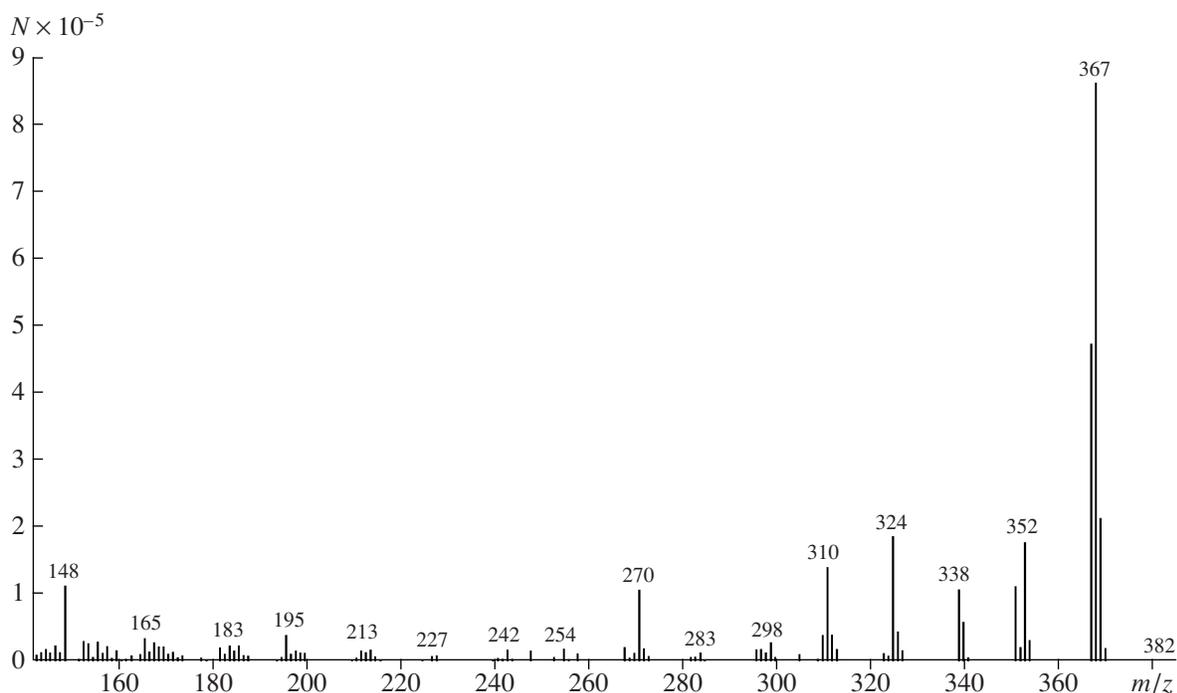
Fig. 6. Mass spectrum of the trifluoroacetyl derivative of desomorphine (retention time, 11.854 min).
