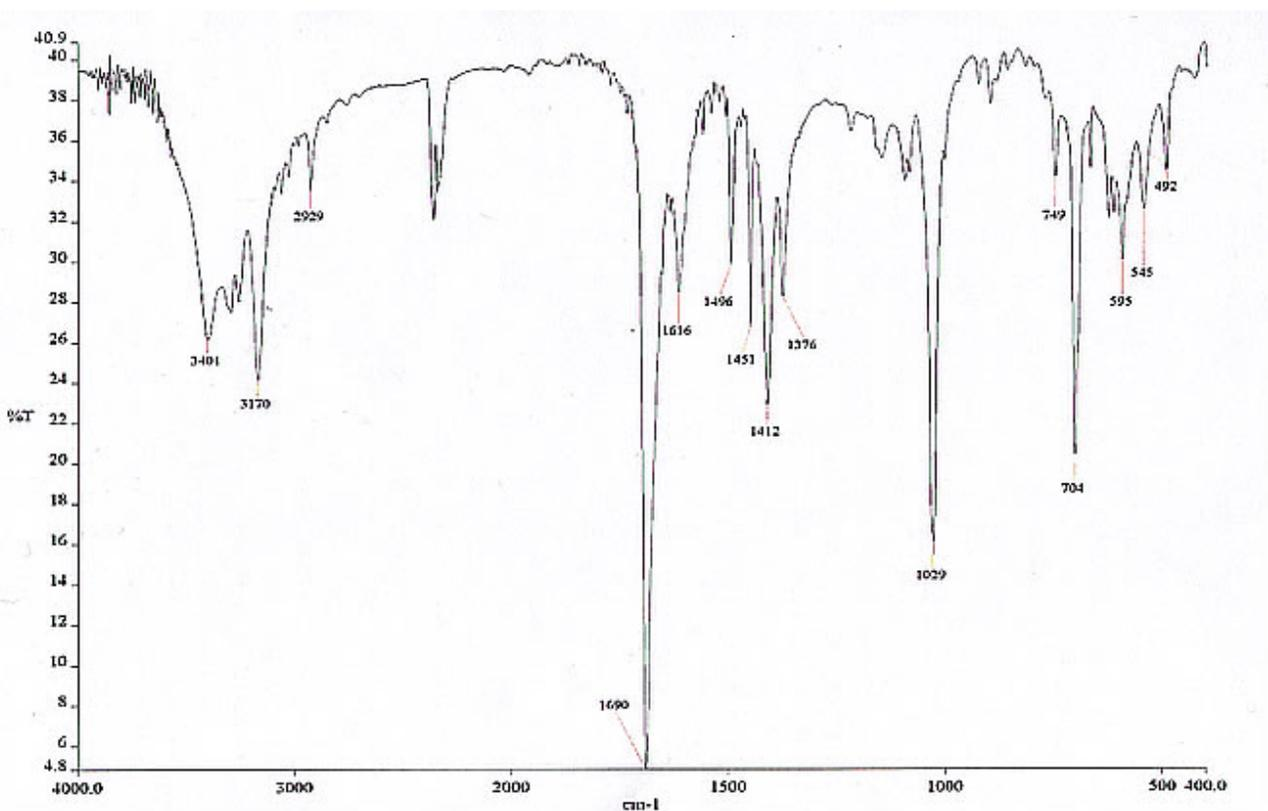
**Figure 4 – Infrared Spectrum of Extracted Modafinil**
