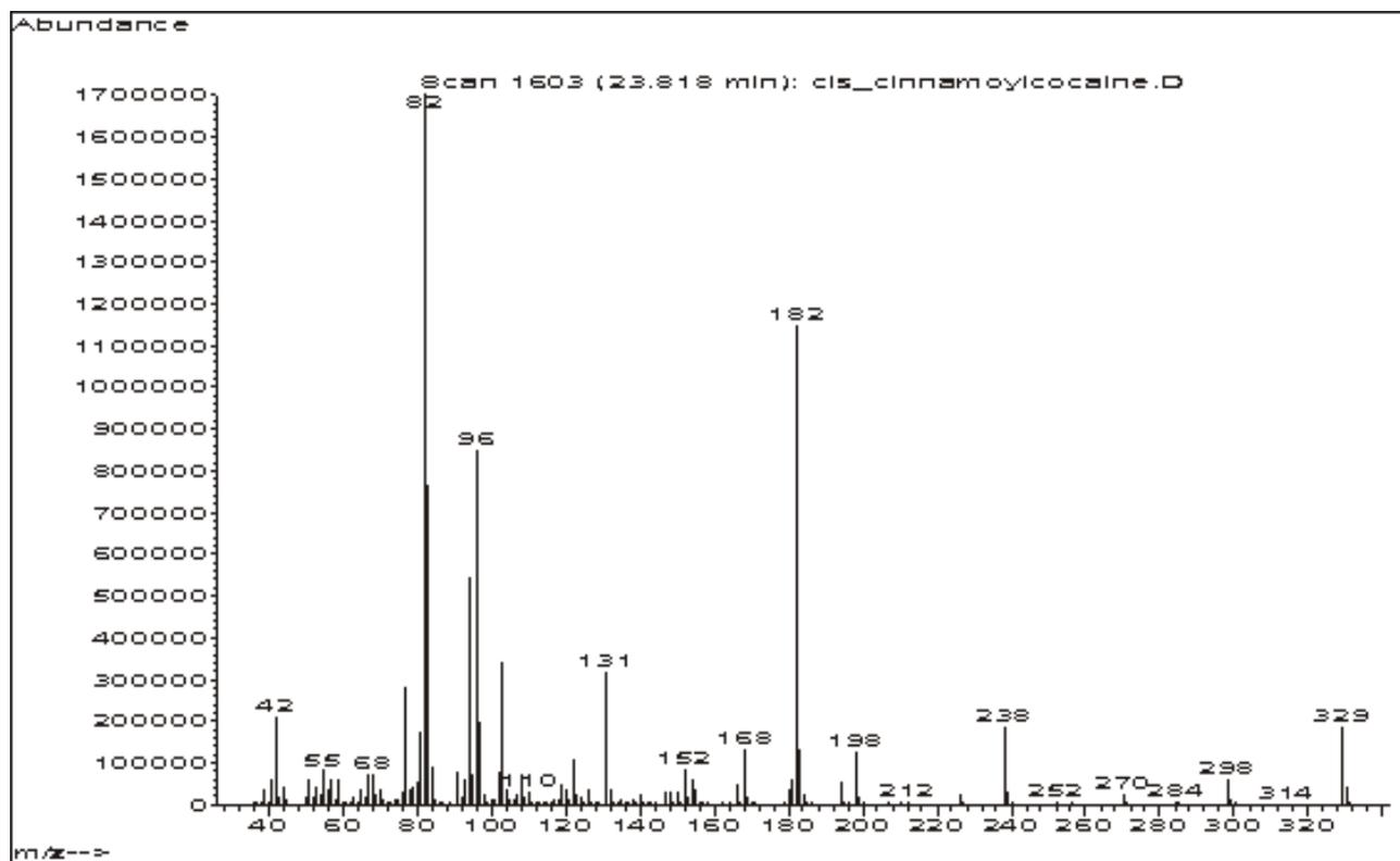
Figure 4. Gas Chromatography/Mass Spectra (70 eV EI) of *cis*-Cinnamoylcocaine.
